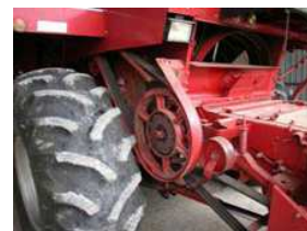
Moving devices without protection
