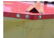
Protection sheet linked with screws to the metallic frame
